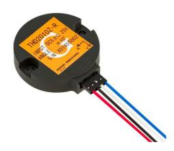
THD2000Z-Series industrial inclinometers are high performance sensors used MEMS accelerometer to determine inclination in X and Y axes with excellent precision. THD2000Z is compact size and it has high vibration resistance.
