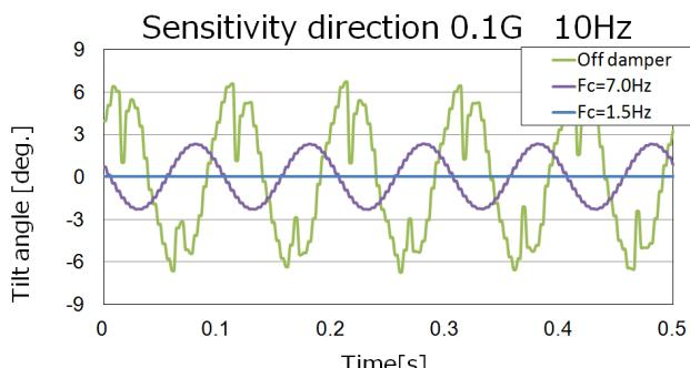
ESC3000Z series implements the digital filter that would remove external noise to give the user a choice of certain filter factor from 16 available settings.
