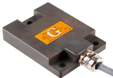
ESC-Series industrial inclinometers are high performance sensors used MEMS accelerometer to determine inclination in X and Y axes with excellent precision. Using Aluminum Die-Cast housing, the versions offer mechanical stability and
